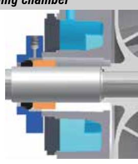
**B (S) gland packing (with flushing)**
